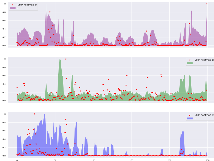
Figure 4.17: Rescaled values of fluid velocity u (upper panel), height h (middle panel), rain r (lower panel) and corresponding LRP heatmaps \alpha (red stars) of u, h, r against all 250 grid points for a single experiment
