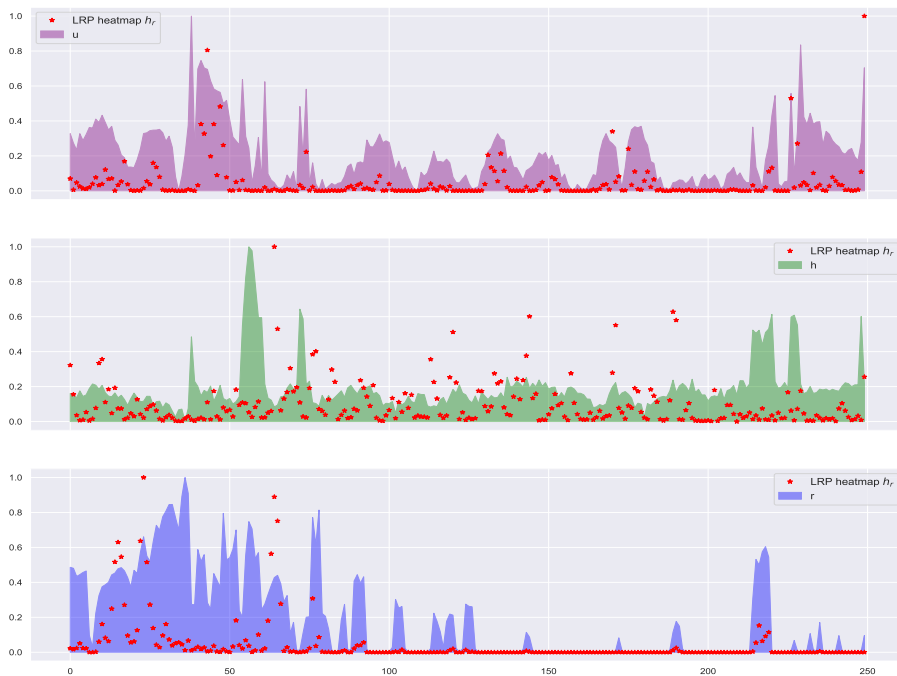
Figure 4.19: Rescaled values of fluid velocity u (upper panel), height h (middle panel), rain r (lower panel) and corresponding LRP heatmaps h_r (red stars) of u, h, r against all 250 grid points for a single experiment
