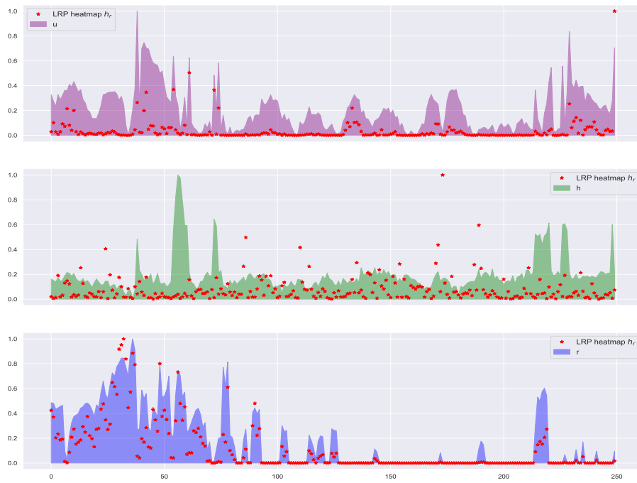
Figure 4.24: Rescaled values of fluid velocity u (upper panel), height h (middle panel), rain r (lower panel) and LRP heatmap h_r (red stars) of u, h, r against all 250 grid points for a single experiment of 3 individually trained NNs
